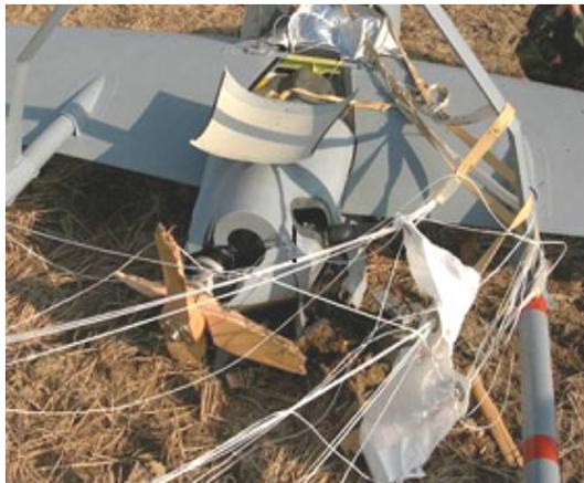
Fig. 6. Aircraft damage situation
