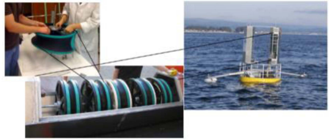
Figure 11. Dielectric elastomer marine wave generator based on articulated dielectric elastomer roll transducer (top left), connected roll of generator module (bottom left) and sea tests (right). 35
