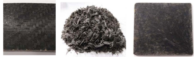
Fig. 4. Recycling test results of carbon fiber polyamide 6 composites (left: CF-PA6 plate, center: after shredding, right: after remelting and remolding)
