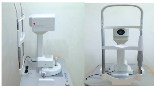
Fig. 3. Photograph of the thermal camera (KR Patent. 10-1662775)
