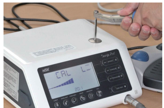
Fig. 1. Calibration for the implant handpiece system.
