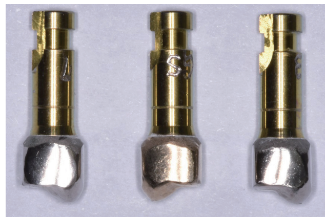
Fig. 1. Cast crown specimens (from left to right): Co-Cr, gold, and Ni-Cr alloys.
