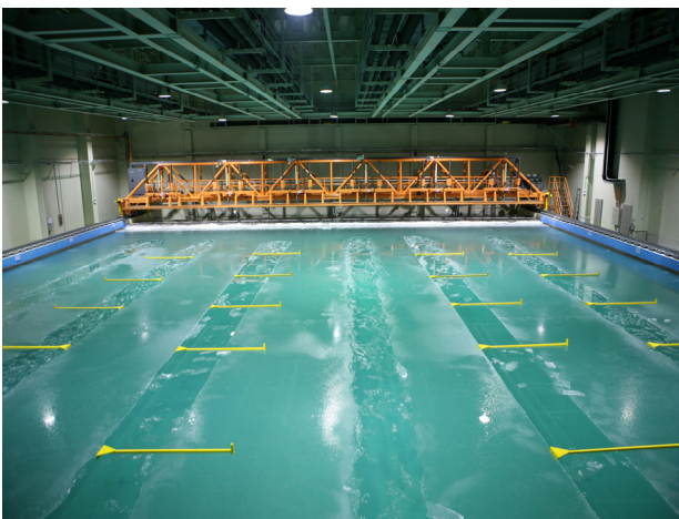
Fig. 3 Photo of KRISO ice model basin
