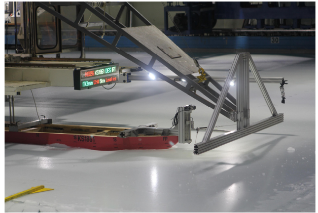
Fig. 5 Bow towing test in level ice
