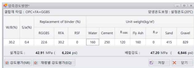
Figure 8. Example of output window of compressive strength
