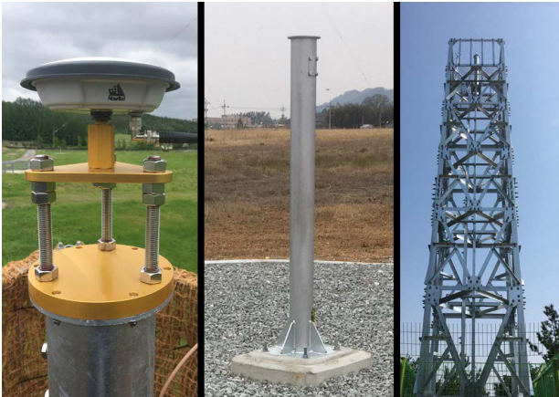
Fig. 6. GPS adapter, steel pipe, steel tower.
