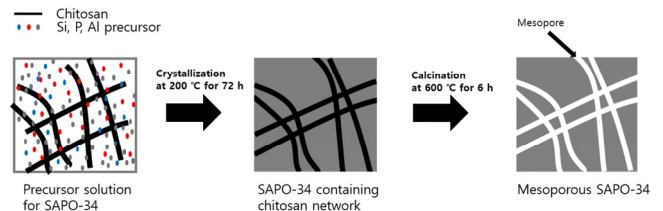
Figure 5. The proposed routes for mesopore formation in a SAPO-34 catalyst.
