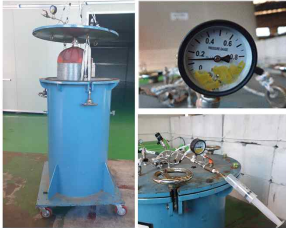
Fig. 11 Hydrogen tank leak test
