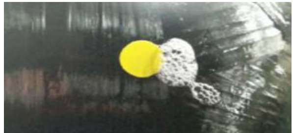
Fig. 9 Bubble formed by penetration of hydrogen gas
