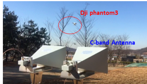
Fig. 4 Doppler detection experiment using C-band radar
