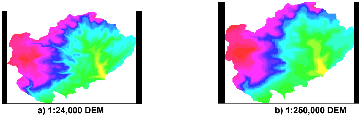
Figure 2. Two DEM images which were used for sensitivity analysis of runoff volumes to model hydrological processes to the choice of cell size; a) is 1:24,000 DEM (7.5-minute) with higher resolution image and b) is 1:250,000 DEM (1-degree) with lower resolution image.
