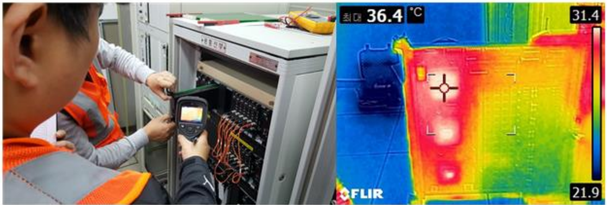
Figure 1. process of thermal imaging of real PCB modules
