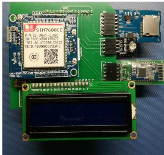
Fig. 4. The final assembled product works successfully with the PCB. The ratio of photo is 1:1
