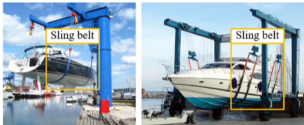
(b) Sling belt for lifting boats (Kim et al., 2019)
