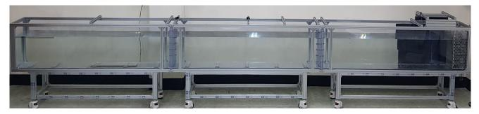
Fig. 2 Overview of Two-dimensional mini wave tank
