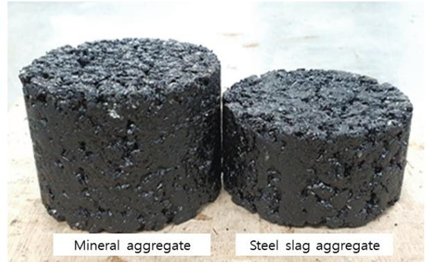
Fig. 1. Volume comparison of specimens using steel slag aggregate and mineral aggregate
