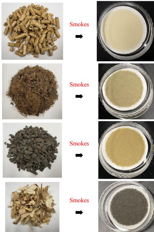
Figure 2. Photographs of raw biomass materials and their smoke samples. Four different biomass materials used in this study are (a) pellet, (b) palm fruit fiber (PFF), (c) PKS, and (d) sawdust.
