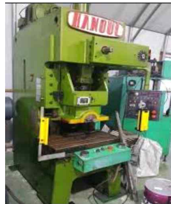
Fig. 1 Press used in the experiment(C type, 35TON)
