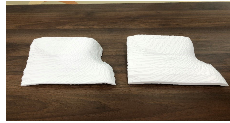
Fig. 4. Produced 3D Bolus(5mm) and 3D Bolus(1cm)
