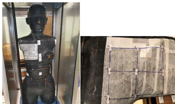
Fig. 1. Dummy Phantom(Rando) with 9 dose measurement points
