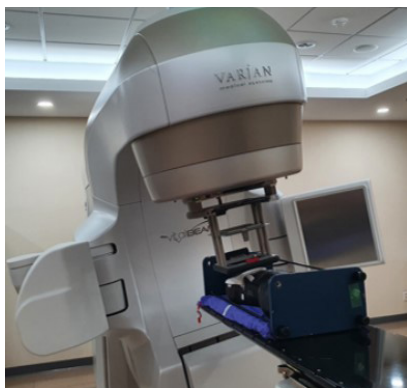
Fig. 7. Dose measurement of Rando Phantom with 3D Bolus
