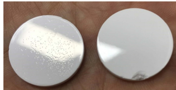
Fig. 6. Digital photographs of macroporous supports with an intermediate α-Al 2 O 3 layer coated by the proposed coating approach without water impregnation (left) and with water impregnation (right).
