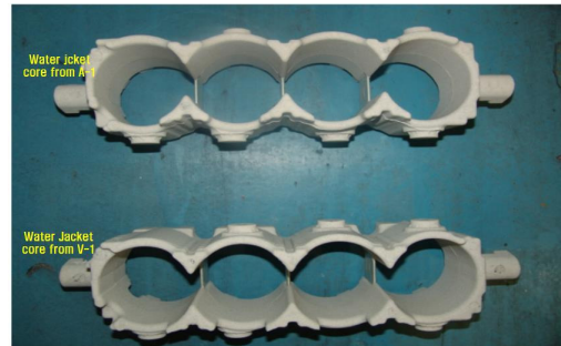
Fig. 9. Two types water jacket core prepared from V-1 and A-1 raw sand
