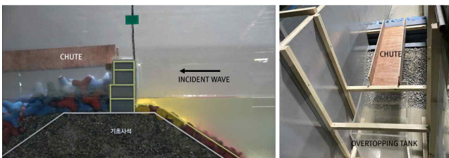
Fig. 4 Installation of chute and tank for measuring wave overtopping
