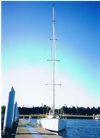
Fig. 1. Titan Lady - a sailing cruiser custom built entirely of titanium
