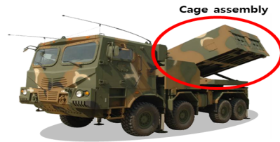
Fig. 2. Cage assembly of K-MLRS Launcher
