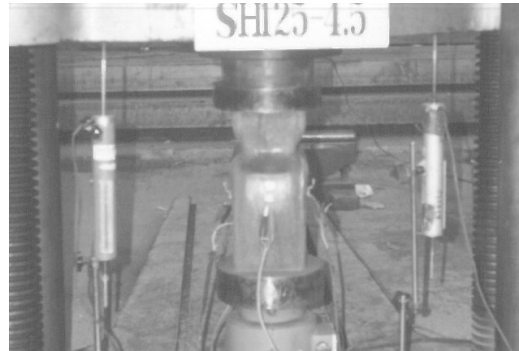
Fig. 6. Local buckling of a hollow steel tube
