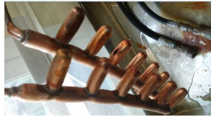
(a) Burst pressure test of finger
