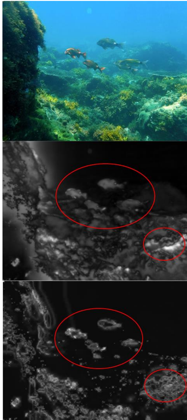
Fig. 4. Input image (top), original saliency map image (middle) and proposed saliency map (bottom)
