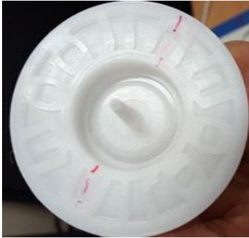
Fig. 5 Roller molding from the mold cooled with low temperature coolant
