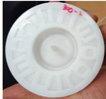
Fig. 8 Roller molding from the mold cooled with high temperature coolant
