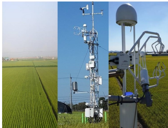
Fig. 1. The map of the study site and the eddy covariance flux measurement tower in the rice paddy in Gimje, South Korea.
