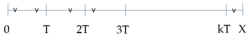
[Figure 1] Shocks arrive(v) randomly and system is replaced at intervals of T until the end of horizon( x )
