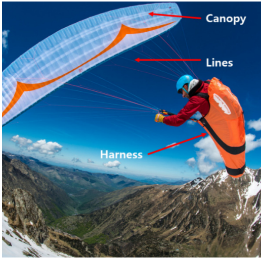
Fig. 1. Components of a paraglider.
