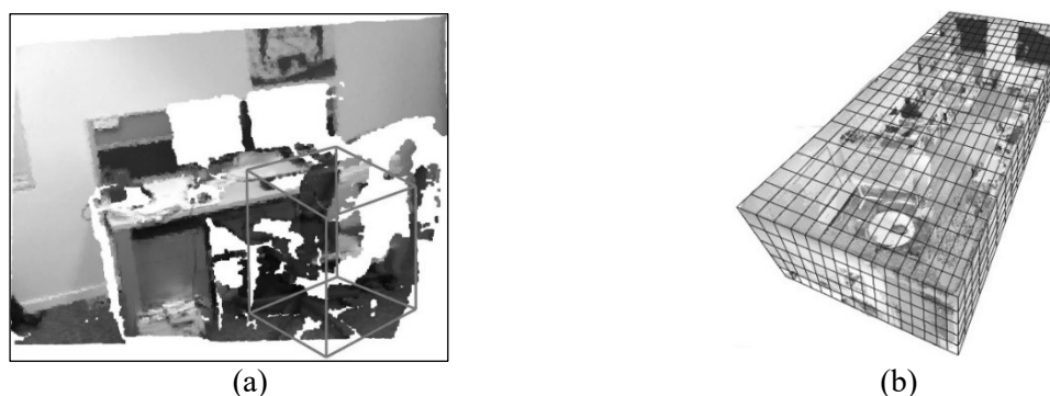
Figure 3. The architecture of the proposed approach. It has two main components: (a) a cuboid proposed in a point cloud, and (b) a voxel labeling database composed of box coordinates of objects
