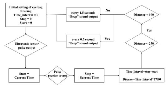
Figure 9. Ultrasonic sensor algorithm
