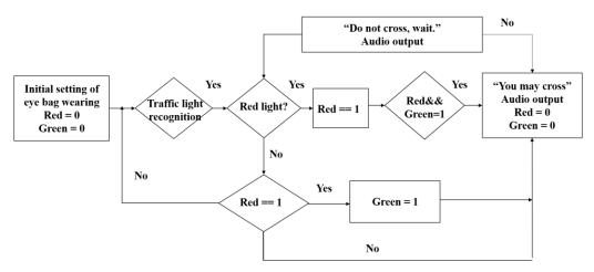
Figure 8. Traffic light algorithm
