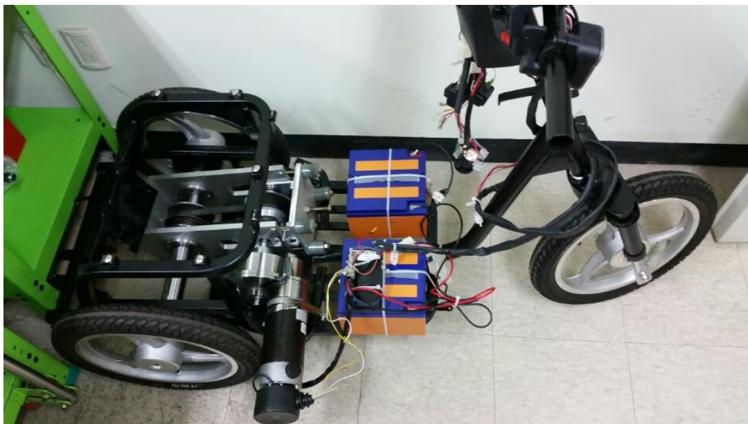
Figure 4. A small electric vehicle equipped with the first CVT model prototype
