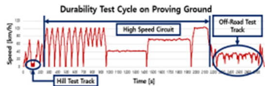
Fig. 6 Test cycle of driving test on the proving ground
