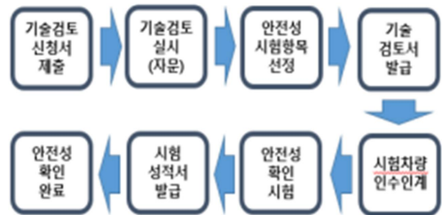
Fig. 3 Procedure of safety test
