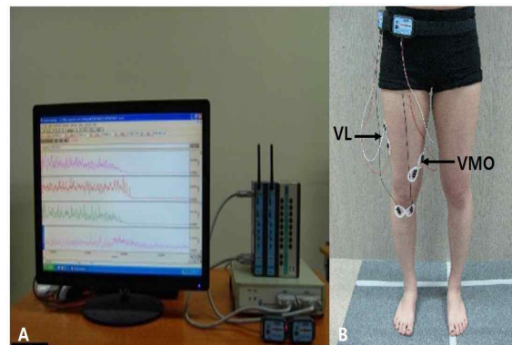
Figure 1. Measurement of muscle activity: A. surface electromyography, B. Placement of surface electrodes(VL; vastus lateralis, VMO; vastus medialis oblique)
