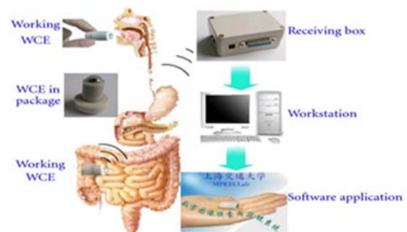
Fig. 1 Wireless Capsule endoscope system.
