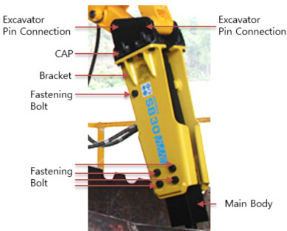
Fig. 3 Picture of a hydraulic breaker without anti-vibration rubber
