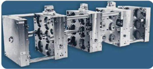
[Figure 1] Injection mold example
