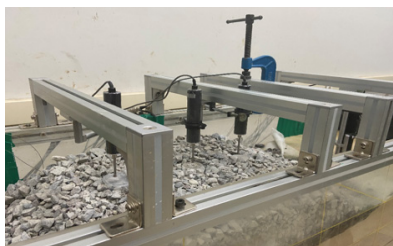
(5) Embankment and LVDT installation
