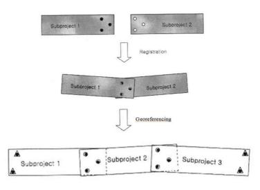
FIGURE 2. The diagram of registration and georeferencing of continuous scan data
