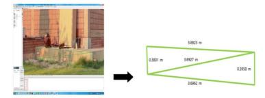
FIGURE 11. Measurement of point-to-point distance from 3D model
