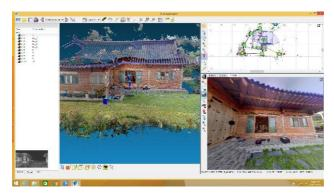
FIGURE 7. 3D model created based on the scan data of St.1
