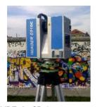
FIGURE 1. 3D Laser scanner (Model: Z+F IMAGER 5010C)
