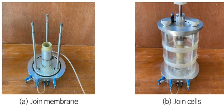
Fig. 3. Process of making test specimen for repeated triaxial compression test.
