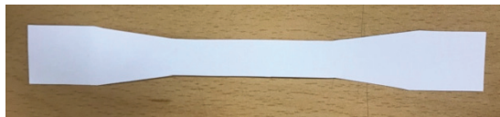
Fig. 3(b). The tensile strength test specimen made 3D printing.
