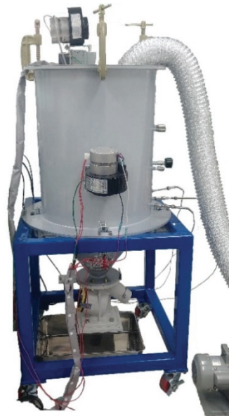
(c) Real image of microwave hopper dryer
