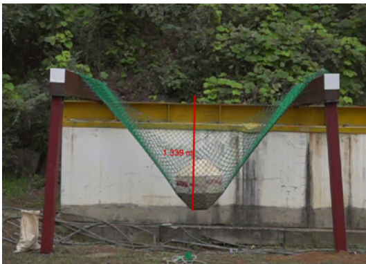
Fig. 5. Final displacement (25kJ)
