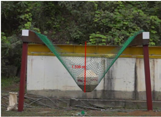
Fig. 4. Instantaneous maximum displacement (25kJ)
