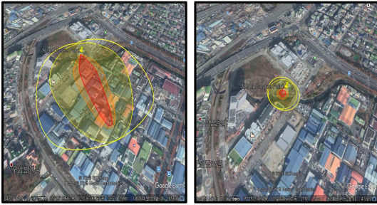
Fig. 8. The distance of overpressure by VCE in C hydrogen station (left : worst case, light : alternative release)
