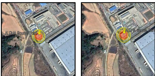
Fig. 5. The distance of radiant heat by Jet fire in A hydrogen station (left : worst case, light : alternative release)
