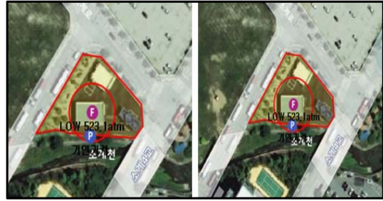
Fig. 9. The distance of radiant heat by Jet fire in C hydrogen station (left : worst case, light : alternative release)
