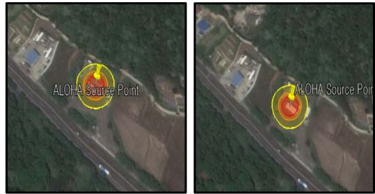
Fig. 7. The distance of radiant heat by Jet fire in B hydrogen station (left : worst case, light : alternative release)
