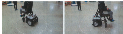
Fig. 10. Rotation radius of moving and lifting wheelchair
