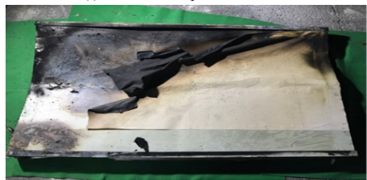
(h) Urethane foam panel backside
