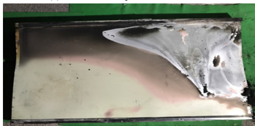
(g) Urethane foam panel heat section
